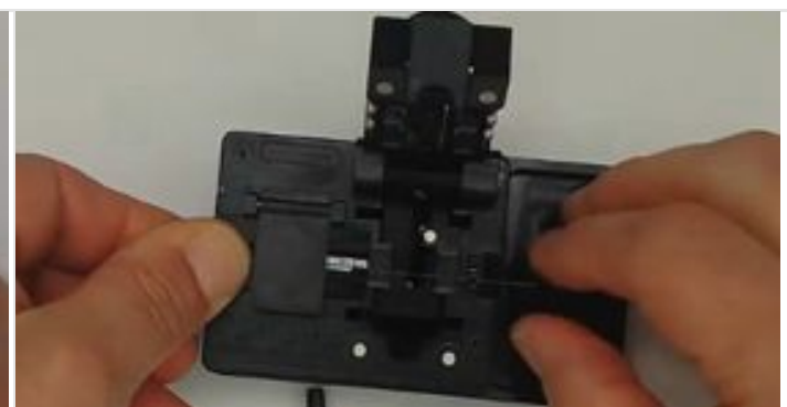
Using fiber cleaver, cut fiber to 12.5mm
